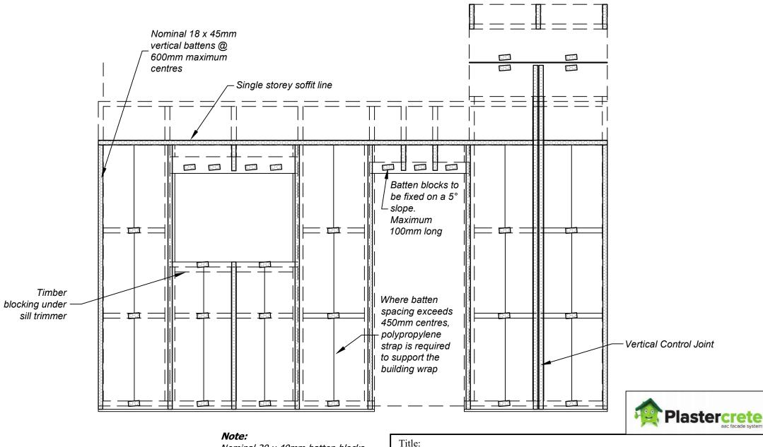
Nominal 20 x 40mm batten blocks 100 maximum may be used providing a minimum of 50mm clearance is left between members
